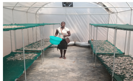
Solar-Biomass Hybrid Dryer installed at Dunga, Kisumu County.
